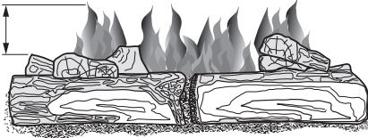
Figure 28 - Correct Burner Flame Pattern
