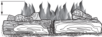
Figure 32 - Correct Burner Flame Pattern
