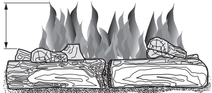
Figure 33 - Incorrect Burner Flame Pattern
