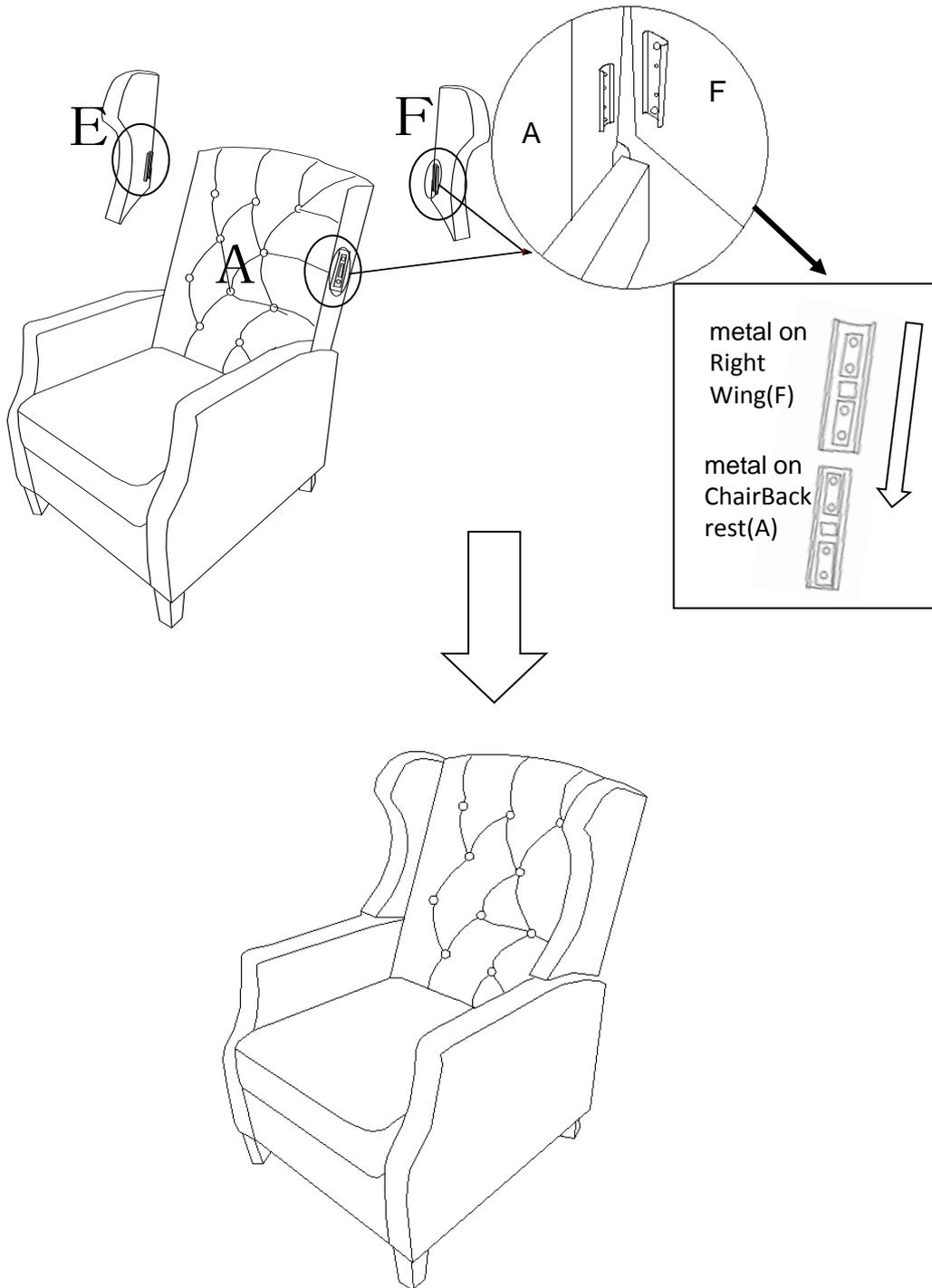
Insert the small metal on the sides of the Left and Right Wing(E)(F) into the prefabricated slide lock gadget on the Chair Backrest(A) as shown above.
