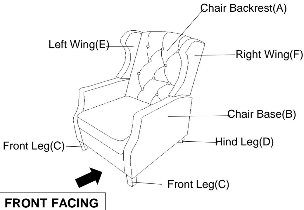
This Push Back Chair has multiplied parts and may require up to some 30 minutes to assemble. To give you an overview of the Push Back Chair parts, the above picture is to help you put the various parts into perspective. Please read through the instructions below to familiarise yourself with the parts and steps before assembly.
