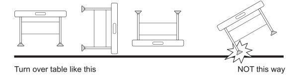
Table may become damaged if it is placed to the floor in an angle.
