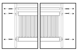
Unscrew the 6 machine bolts **K** and barrel nuts **L** and remove the cross bar **P** and stationary side **B**.
