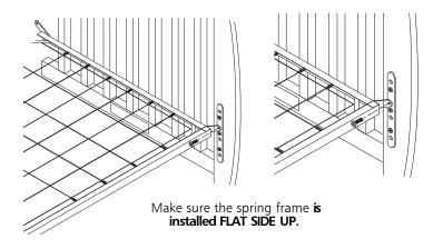
Swing out four hangers at corner of the spring frame **G** carefully. Attach spring frame **FLAT SIDE UP**. Choose the height of the spring frame. Start at the highest level and adjust accordingly.
