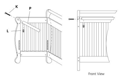
Attach cross bar **P** to the left and right side with 2 machine bolts **K** and 2 barrel nuts **L**. Make sure to insert the cross bar dowel into the correct hole on the left and right legs before inserting the machine holts
