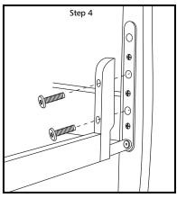
Attach guard rail **Y** to each post bracket on the drop side with 2 allen head bolts **W**.
