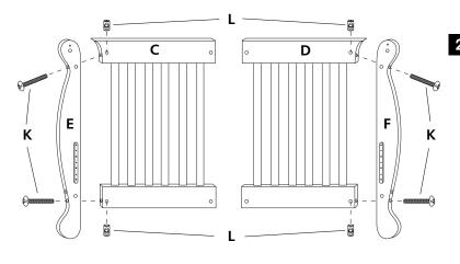
Attach left leg **E** to left side **C** using 2 machine bolts **K** and 2 barrel nuts **L**.
