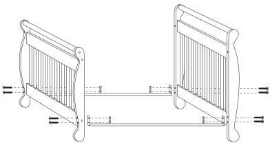
Attach the headboard and footboard assembly with the full size rail conversion kit\* (sold separately). Attach the rails using 8 machine bolts and 8 nuts provided.
