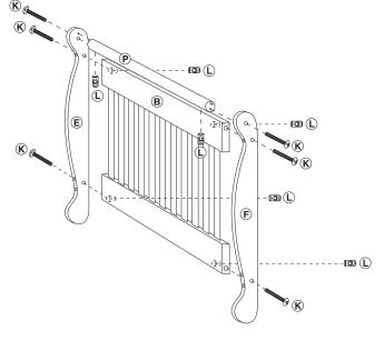
The footboard assembly consists of left leg **E**, right leg **F**, stationary side **B**, and cross bar **P**
