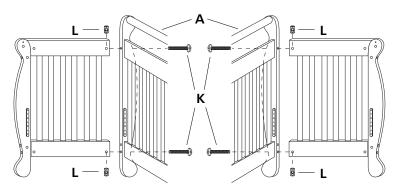
Attach the completed left and ride sides to the headboard **A** using 2 machine bolts **K** and 2 barrel nuts **L** for each headboard.
