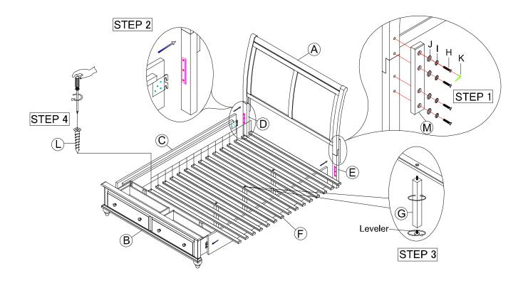
STEP 1: Attach the Left and Right post(D&E) to the Headboard(A) using the Flat Washer(J),
