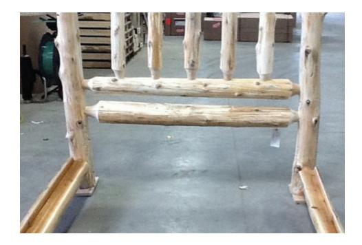
6. Lightly screw the lag screws with washers into the headboard and footboard into the side rails. Do not tighten the lag screws at this time. Hint: Scrape the lag screws across a bar of soap or wax to make it easier to install them. Re-check position of the rails so that they match the photo above.
