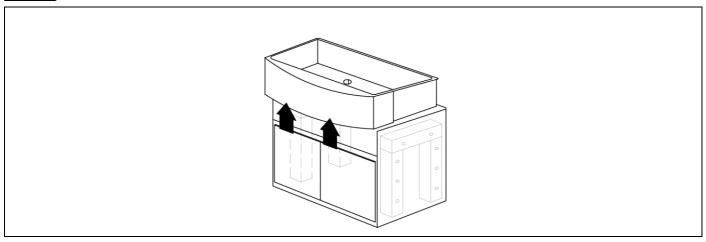
Step 7: Apply the silicone sealant to the top of each support.
