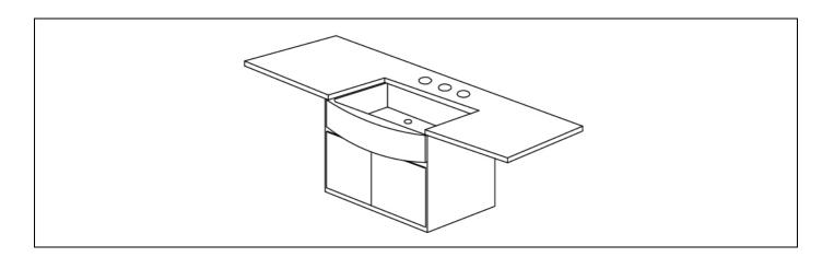
Step 10: Install the secure clips to the countertop, make sure each clip engages with the rim of the sink (minimum 4 clips in back, 2 clips per side). Tighten each clips evenly.
