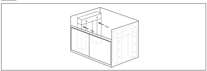
Step 5: Put the sink into the cabinet. Check if the sink is resting on the supports.
