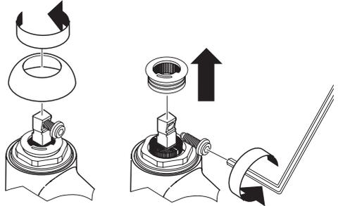
Replace the high temperature limit stop so that the pin on the cartridge is in the desired slot on the limit stop. Note: the temperatures given in the diagram assume a water heater temperature of 140° F, a cold water temperature of 50° F and a water pressure of 45 PSI.
