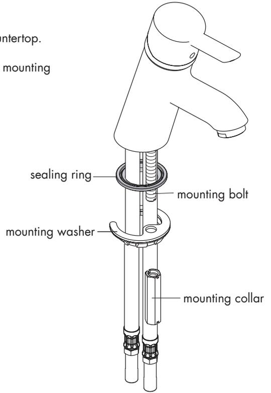
Attach the hoses to the supply stops with 3/8" compression fittings (not included). Use two wrenches, as shown, to prevent the hoses from twisting or from becoming loose.
